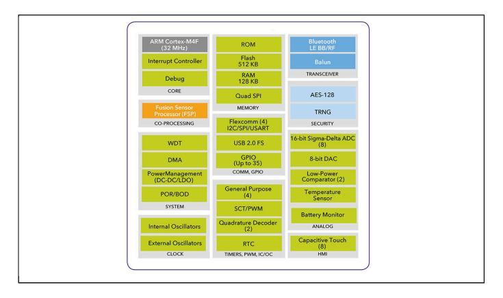
View additional information for QN908x: Ultra-Low-Power Bluetooth Low Energy System on Chip Solution.
