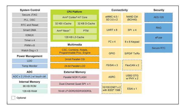
View additional information for i.MX 6ULL Single-Core Processor with Arm® Cortex®-A7 Core.
